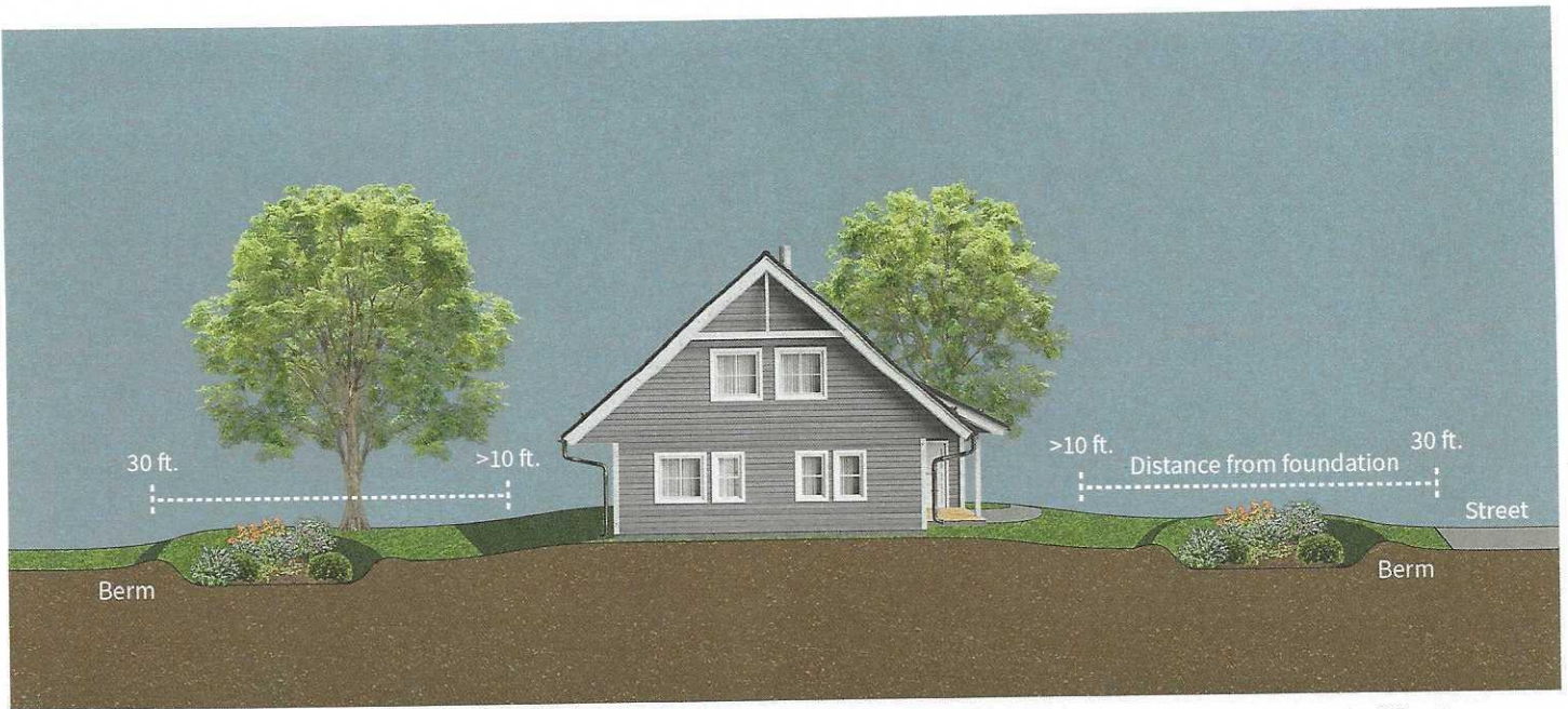
Figure 2. Rain gardens should be placed at least ten feet from the house and within thirty feet from the mouth of the downspout. Ideally, they should also be situated on a gentle slope that catches downspout water.
